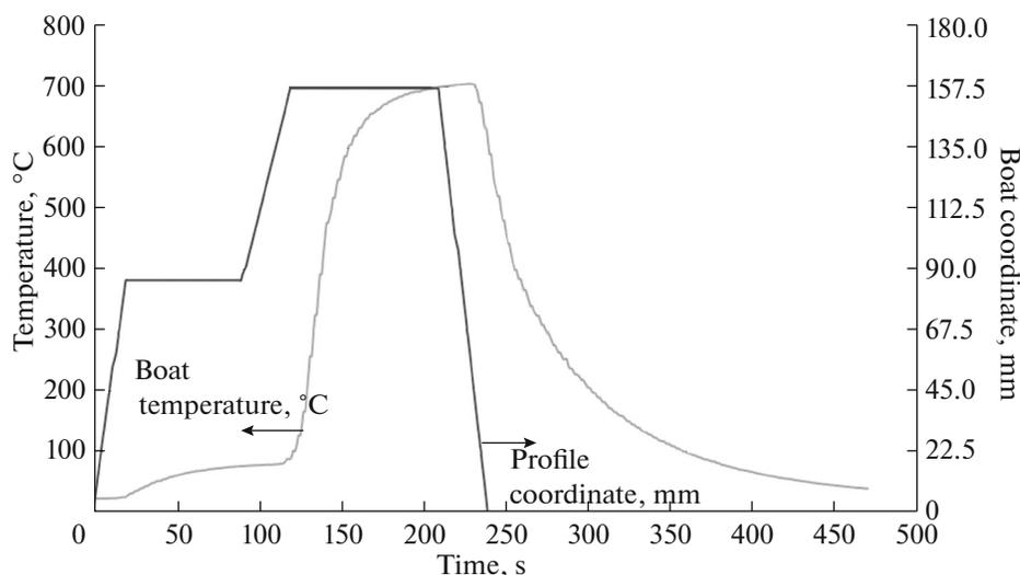
Fig. 2. Optimum profile of boat motion and a graph of the dependence of the change in boat temperature on the time of its motion.
